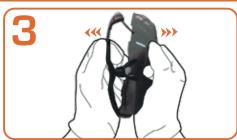
Follow along the frame groove from top to bottom (right to left) to separate the lens from the frame tabs and remove the lens completely.
