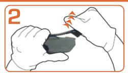
Hold the right temple with your left hand and the right side of the lens with your right hand. Pull the lens outward in the direction of the arrow (pictured) to separate it from the frame.
